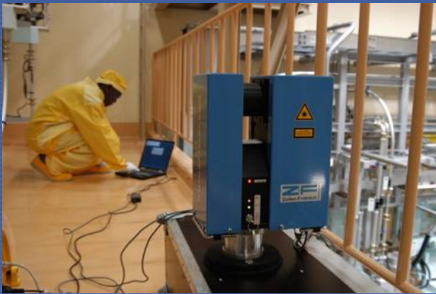
IAEA Inspector performing a 3DLR scan. IAEA SG- JNFL.
